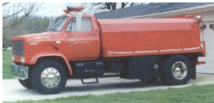
Photo 2: A 2,000-gallon Water Tender with a 300-GPM pump
